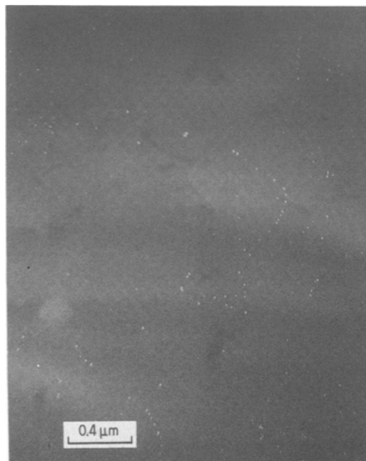
Figure 6 Precipitation of Nb(C, N) in austenite at 675^{\circ} C before the start of transformation.
